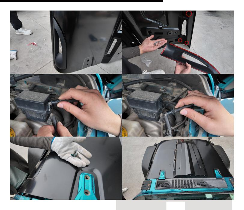
Prepare required components ( $1 \times 1$ ,  $2 \times 1$ ,  $3 \times 6$ ,  $4 \times 6$ ). Adhere 2 to 1 as diagrammed. At red-circled locations, fasten 1 to the hood using 3 and 4.
