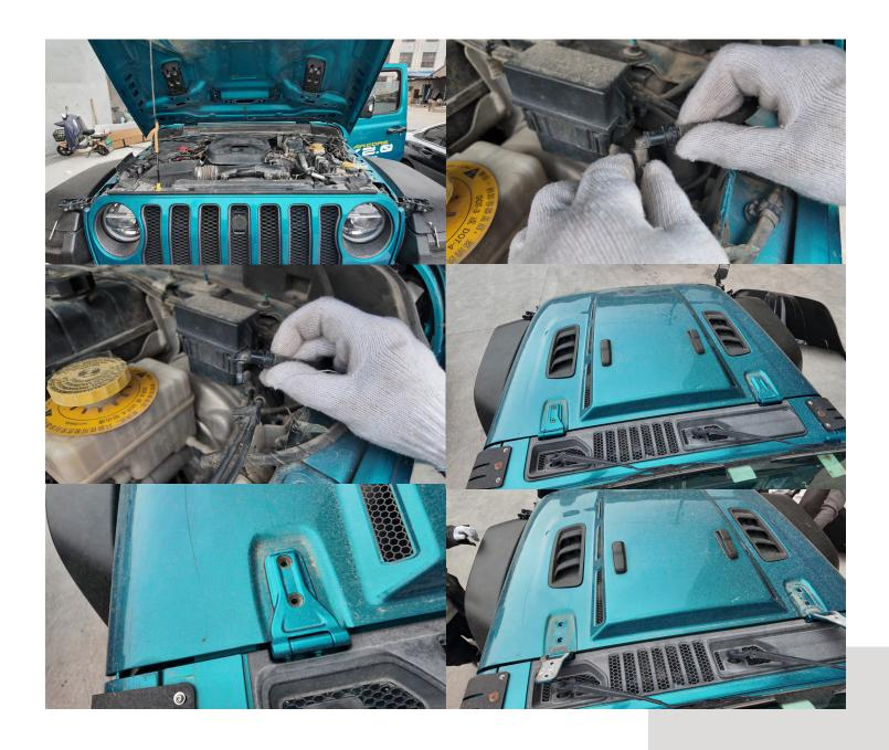
Open the hood, disconnect the washer fluid hose, close the hood, remove the hinge screws, and detach the hood from the vehicle.
