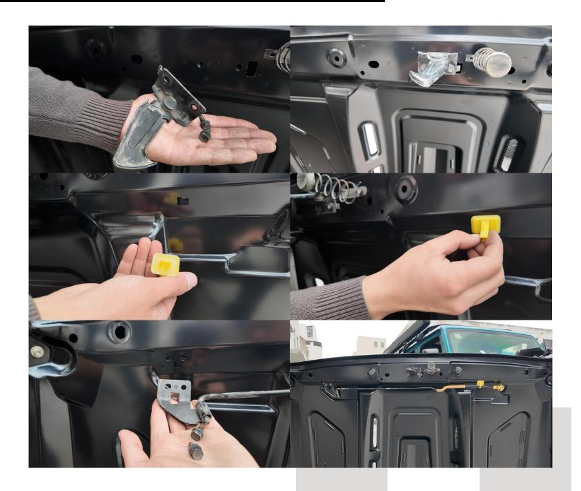
As shown in the diagram, install the original vehicle components onto the new hood.
