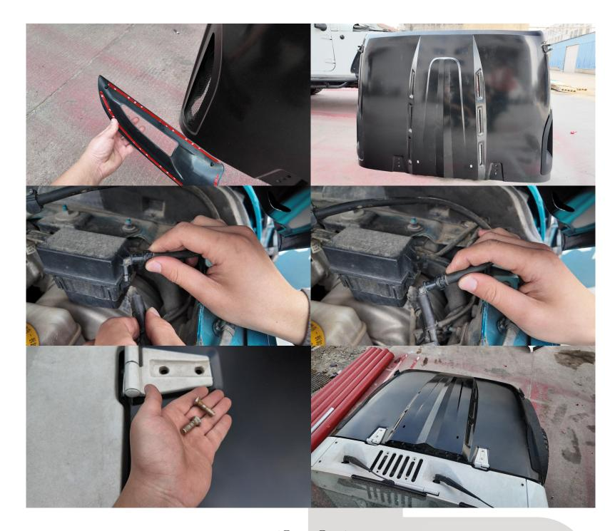
Prepare required components (①×1, ②×1). As shown in the diagram, use ② to install ① onto the hood. Lift the assembled hood onto the vehicle, connect the washer fluid hose, and secure the hood to the hinge with the original vehicle screws
