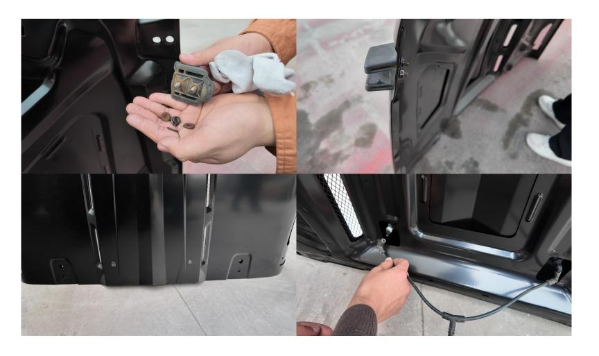
As shown in the diagram, install the original vehicle components onto the new hood.
