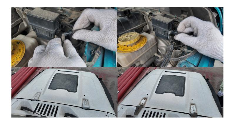
Open the hood, disconnect the washer fluid hose, close the hood, remove the hinge screws, and detach the hood from the vehicle.
