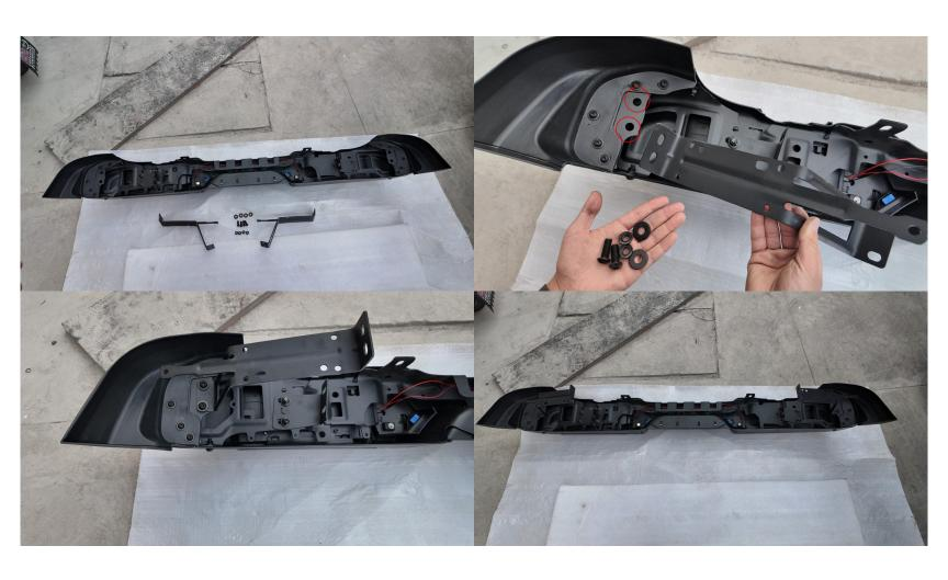
Prepare required parts (①×2, a×4, c×4, d×4). As shown in the diagram, use a, c, d to secure ① to the red circle markings. (Note: Do not tighten.)
