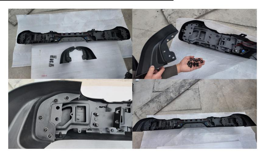
Prepare required parts (3×2 or 4×2, b×10, e×10, f×10). As shown in the diagram, use b, e, f to connect 3 or 4 and the bumper.
