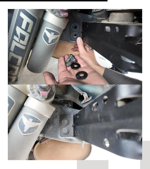
Prepare required parts (d×4). As shown in the diagram, use d and original vehicle screws to secure ① to the vehicle frame at the blue circle markings.
