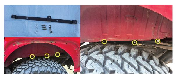
Assemble the necessary components for installing the inner fender liner and position them as shown in the diagram.
