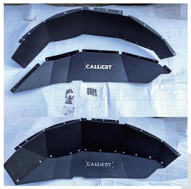
Hardware required. Preassemble the front inner fender liner using bolts, washers, nuts. Leave the bolts finger tight, as they will be tightened in a later step.
