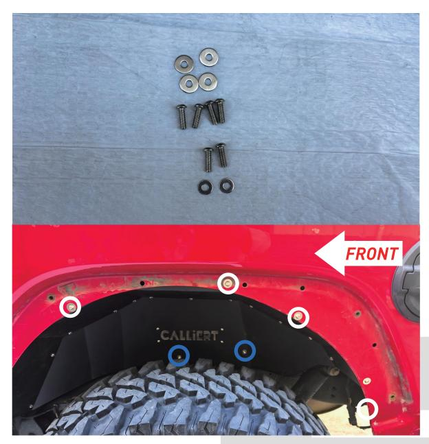
Gather the required components for installing the inner fender and position them as illustrated.
