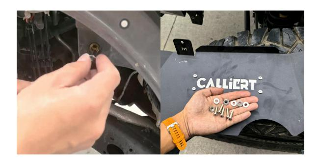
Install the rivet nut into the designed hole. Drilling is necessary to fit the rivet nut into the hole.
