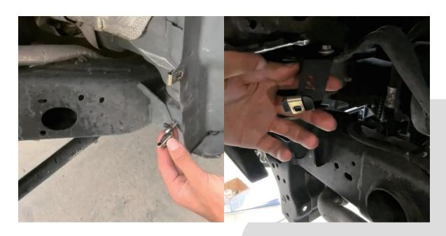
Secure the lower mounting point using the bolts, washers, threaded plate (item no.6). Connected by the clip nut.
