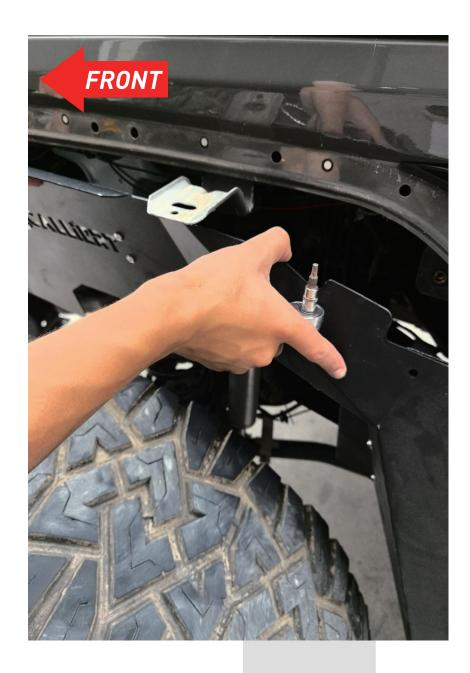
Mounting the pre-assembled liner to the body using bolts, washers and nuts. Next, attempt to tighten all the inner fender bolts that were previously hand tight. Bolt the last bolt through the factory hole.
