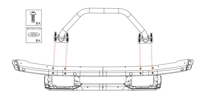
Attention: Remove the screws from the original vehicle before installation. The Upgrade Bull Bar was installed using the original screws removed from the vehicle. Please use the washer provided by us.
