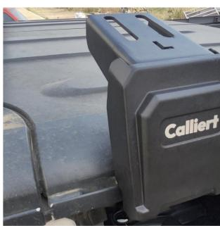
Prepare the required components (E x4). First, loosen the two screws at the bottom of E, then snap E into the rain channel as illustrated.
