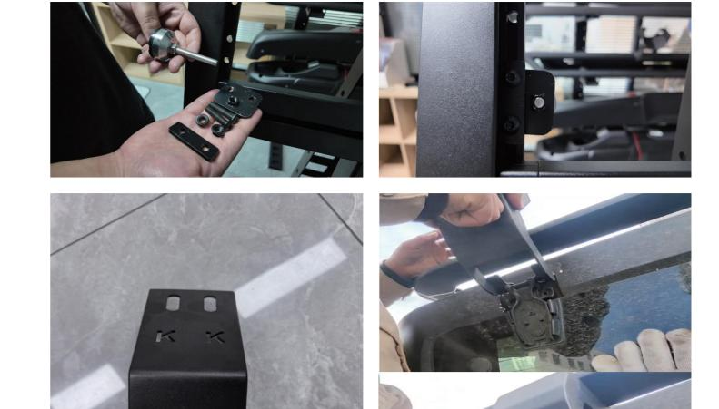
Prepare the required components (G x2, H x2, J x4, M x4, O x2). As illustrated, connect G and D using components G, J, and M, then securely screw O into the threaded mounting holes on G.
