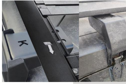
Prepare the required components (E x2). First, loosen the two screws at the bottom of E, then snap E into the rain channel as illustrated.
