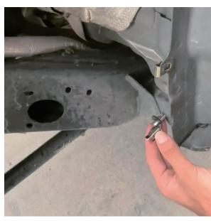
Secure the lower mounting point using the bolts, washers, threaded plate (item no.6). Connected by the clip nut.
