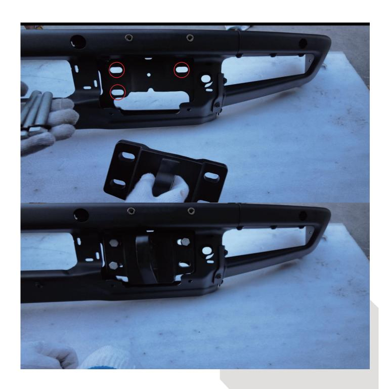
Prepare required components (3\*1, a\*3, b\*3). As shown in the diagram, insert (a, b) through 3 and 9 in red-circled area.
