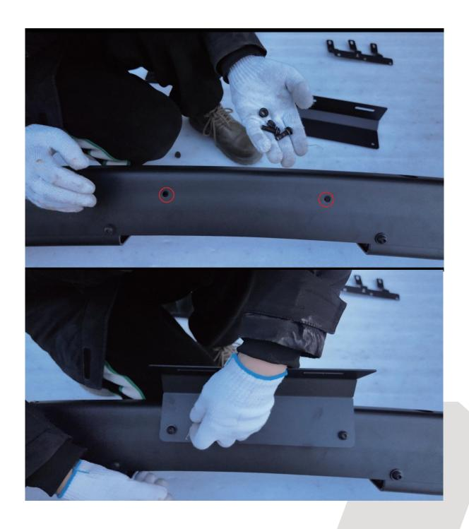
Prepare required components (5\*1, e\*2, f\*2, g\*2, h\*2). As shown in the diagram, connect (1) and (5) in red-circled area using (e, f, g, h).
