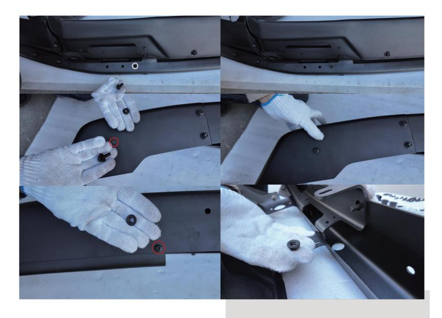
As shown in the diagram, connect 1 and 8 in white-circled area using  $(e,\ f,\ g)$ , then connect 1 and 8 in red-circled area using  $(e,\ f,\ g,\ h)$ .
