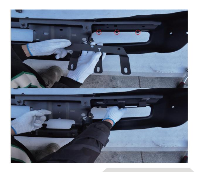
If installing spotlights, as shown in the diagram, remove the screw at red-circled area, then install 6 to red-circled mounting hole using the removed screw.
