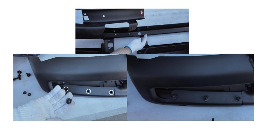
Prepare required components (1\*1, 8\*1, e\*6, f\*6, g\*6, h\*2) . As shown in the diagram, align 1 and 8 at red-circled area, then connect 1 and 8 in white-circled area using (e, f, g) .
