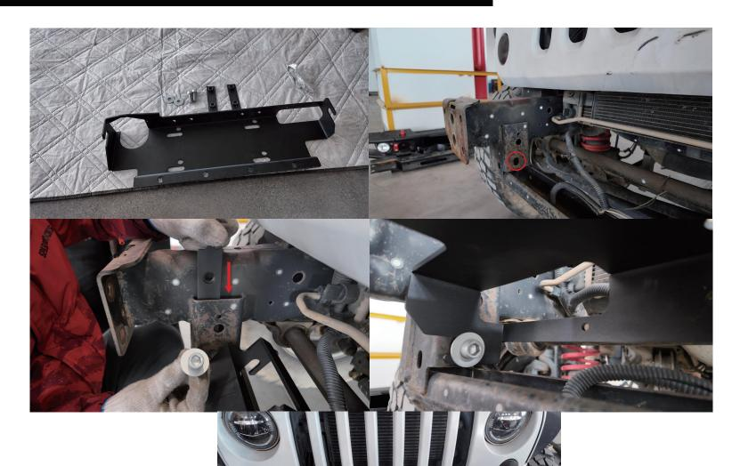
Prepare required components (3\*1, a\*2, d\*2, i\*2). As shown in the diagram, connect 3 and the vehicle beam using (a, d, i).
