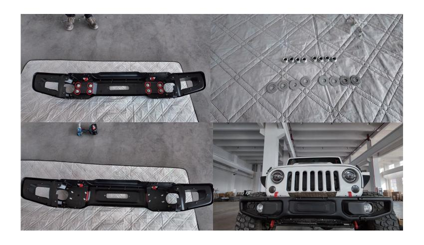
As shown in the diagram, connect the bumper and vehicle beam using screws and washers removed from **(10)**.
