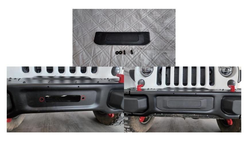
Prepare required components (6\*1, c\*2, j\*2). As shown in the diagram, connect 6 and the vehicle beam using (c, j).
