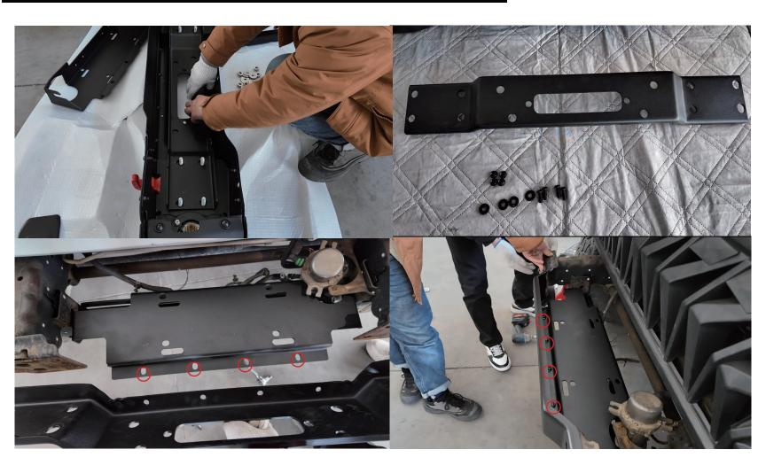
repare required components (c\*4, g\*4, j\*4). As shown in the diagram, first remove 1 from bumper, then connect 1 and 3 at red-circled area using (c, g, j).
