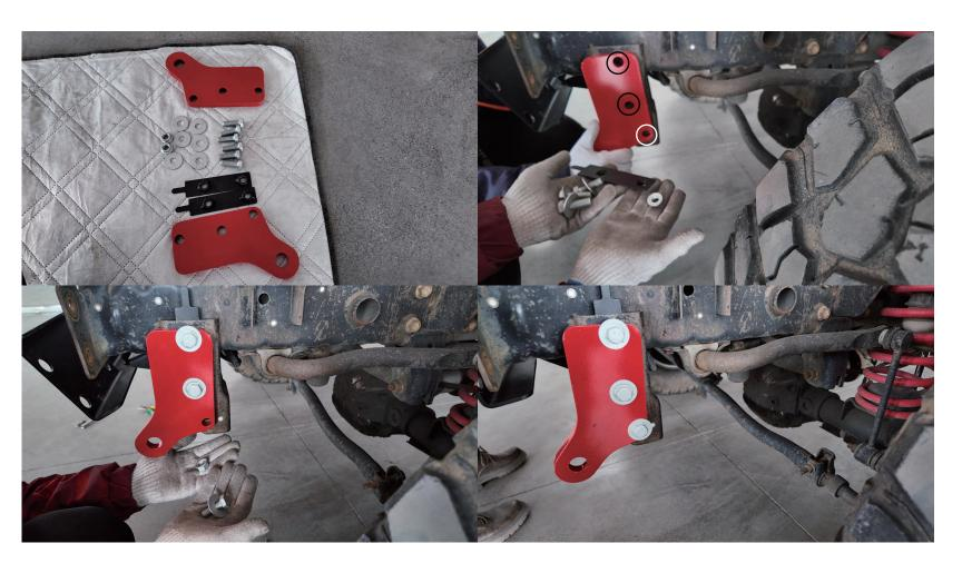
Prepare required components (4\*1, a\*2, e\*6, f\*2, i\*6). As shown in the diagram, using (a, e, i) to connect 4 to the vehicle beam at the black-circle, then using (e, f, i) to connect 4 and the vehicle beam at white-circled
