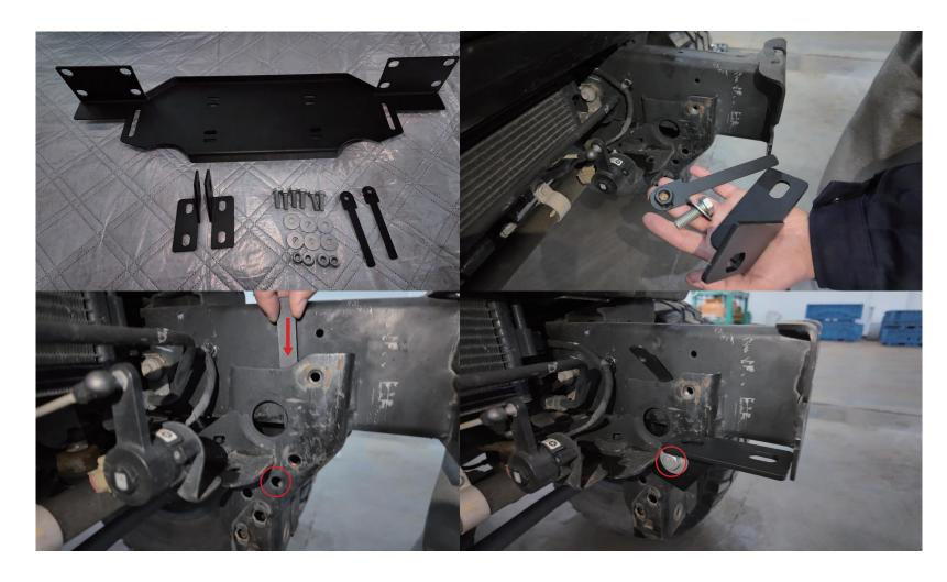
Prepare the following components (2 \*2, 3 \*1, a\*2, e\*6, f\*4, i\*6), As shown in the diagram, connect 2 to the vehicle chassis beam using (a, e, i)
