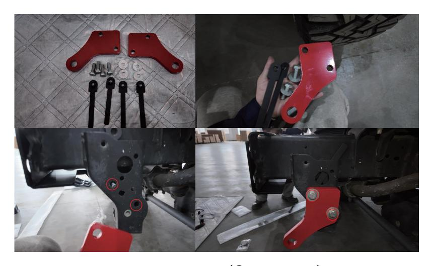
Prepare required components (4\*2, a\*4, e\*4, i\*4). As shown in the diagram, connect 4 to the vehicle chassis beam using (a, e, i).
