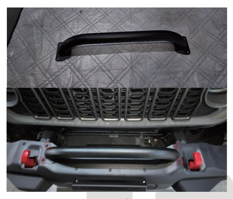
Remove circled screws, then connect (9) to bumper using removed screws.
