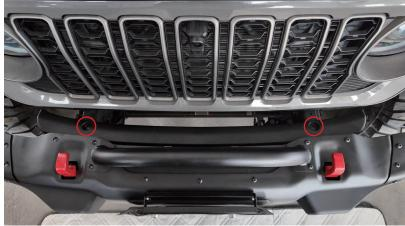
As shown in the diagram, connect (10) to beam at circled holes.
