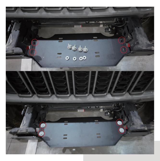
As shown in the diagram, connect 2 to 3 using (e, f, i).
